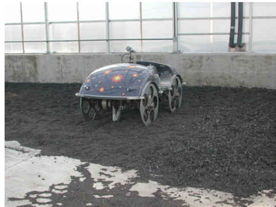
Lisa the Mole, named after the Simpson's character, moves randomly through the greenhouse turning the solids and has sensors to turn when walls are encountered.
